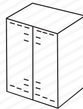
Bottom stitching of regular slotted container.
