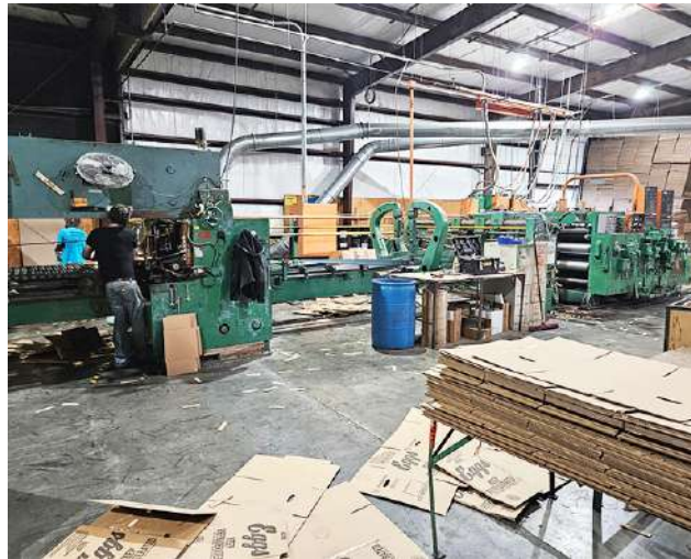
50" x 110" S&S 2-Color Flexo Folder Gluer, Model ZLR
